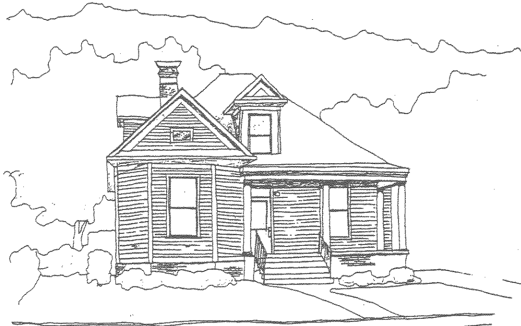
Gabled Ell plan St. Elmo dwelling showing orientation and lot placement (4309 St. Elmo Avenue).
